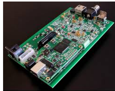
Figure 2. FPGA module installed in an industrial instrument.
